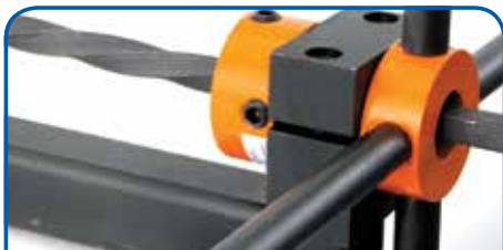
Bar to be twisted is locked in place using the gripping bolts.
