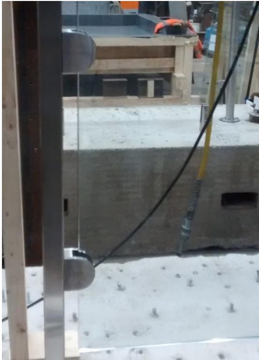
Plate 5 – Test 2a – Timeless Square Posts – 15 mm Toughened Glass – Mixture of Clamp Types
