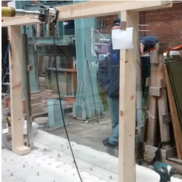
Plate 1 – Test 1a – Timeless Square Posts – 10 mm Toughened Glass – Horizontal Line Load – Load Application Side
