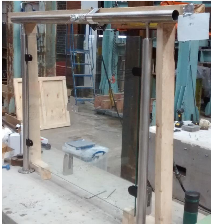
Plate 11 – Test 4a – Timeless Round Posts – 10 mm Toughened Glass – Black Clamps -Horizontal Line Load – Deflection Measurement Side
