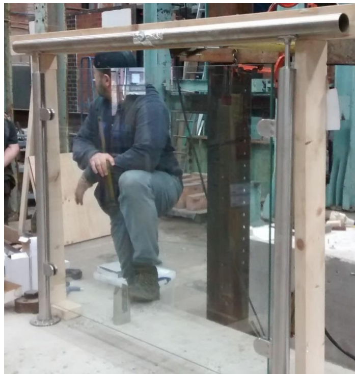
Plate 6 – Test 3a – Timeless Round Posts – 10 mm Toughened Glass – Horizontal Line Load – Deflection Measurement Side
