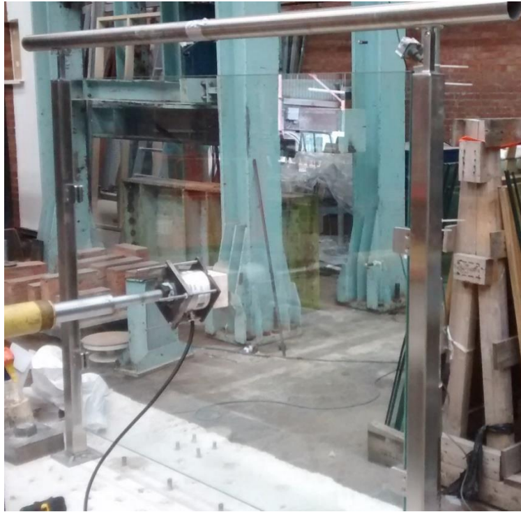
Plate 3 – Test 1c – Timeless Square Posts – 10 mm Toughened Glass – Point Load – Load Application Side
