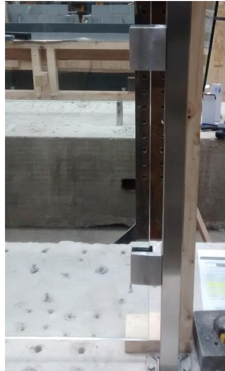
Plate 5 – Test 2a – Timeless Square Posts – 15 mm Toughened Glass – Mixture of Clamp Types
