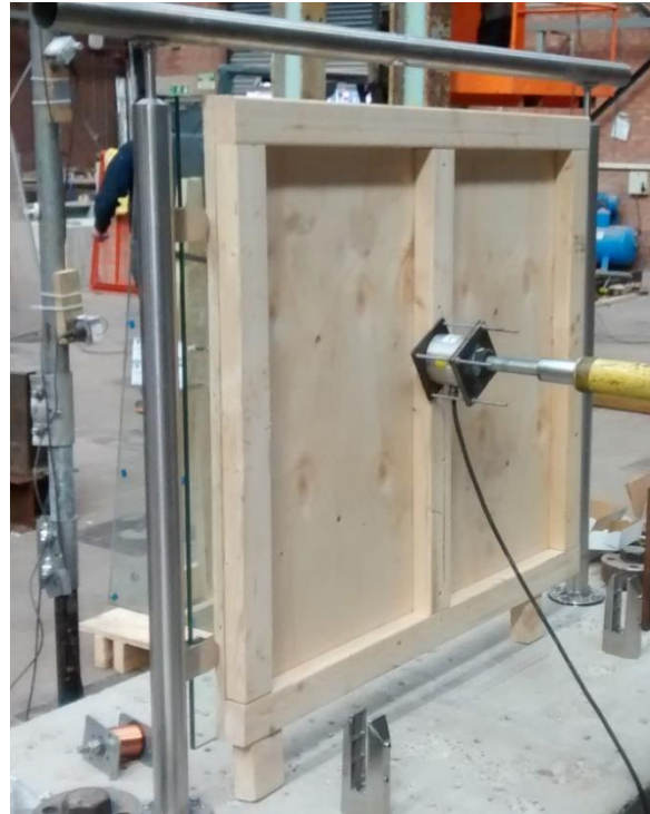
Plate 7 – Test 3b – Timeless Round Posts – 10 mm Toughened Glass – UDL – Load Application Side
