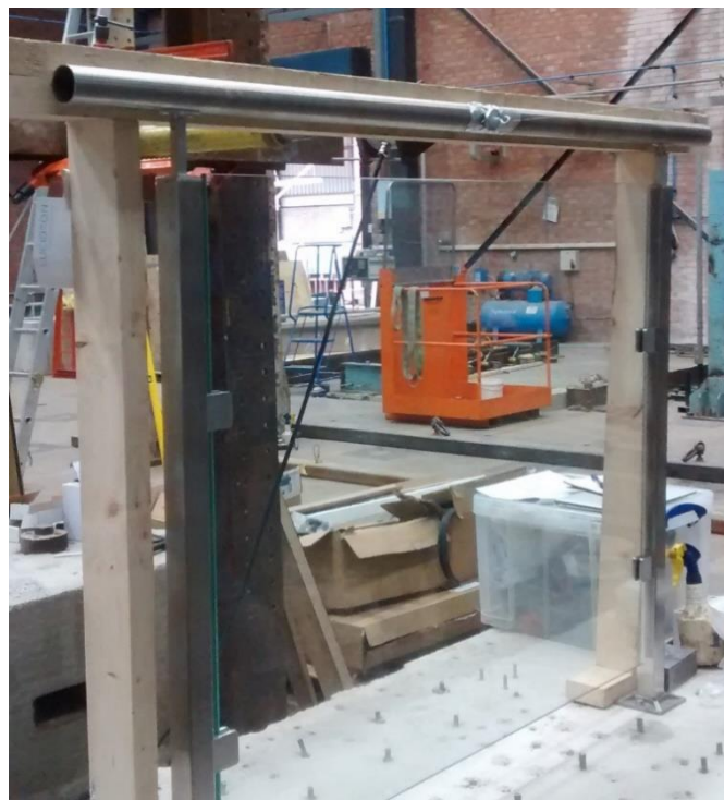
Plate 2 – Test 1a – Timeless Square Posts – 10 mm Toughened Glass – Horizontal Line Load - Deflection Measurement Side
