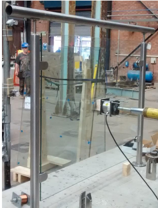
Plate 9 – Test 3c – Timeless Round Posts – 10 mm Toughened Glass – Point Load – Load Application Side
