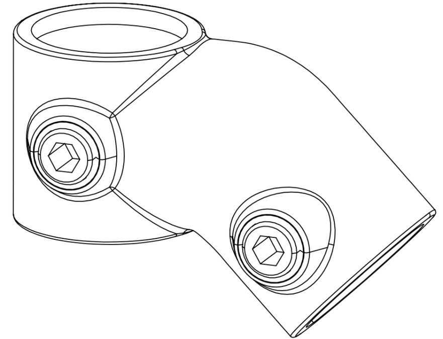
The 45° Tee is used as a bracing and strut component for strengthening structures.
